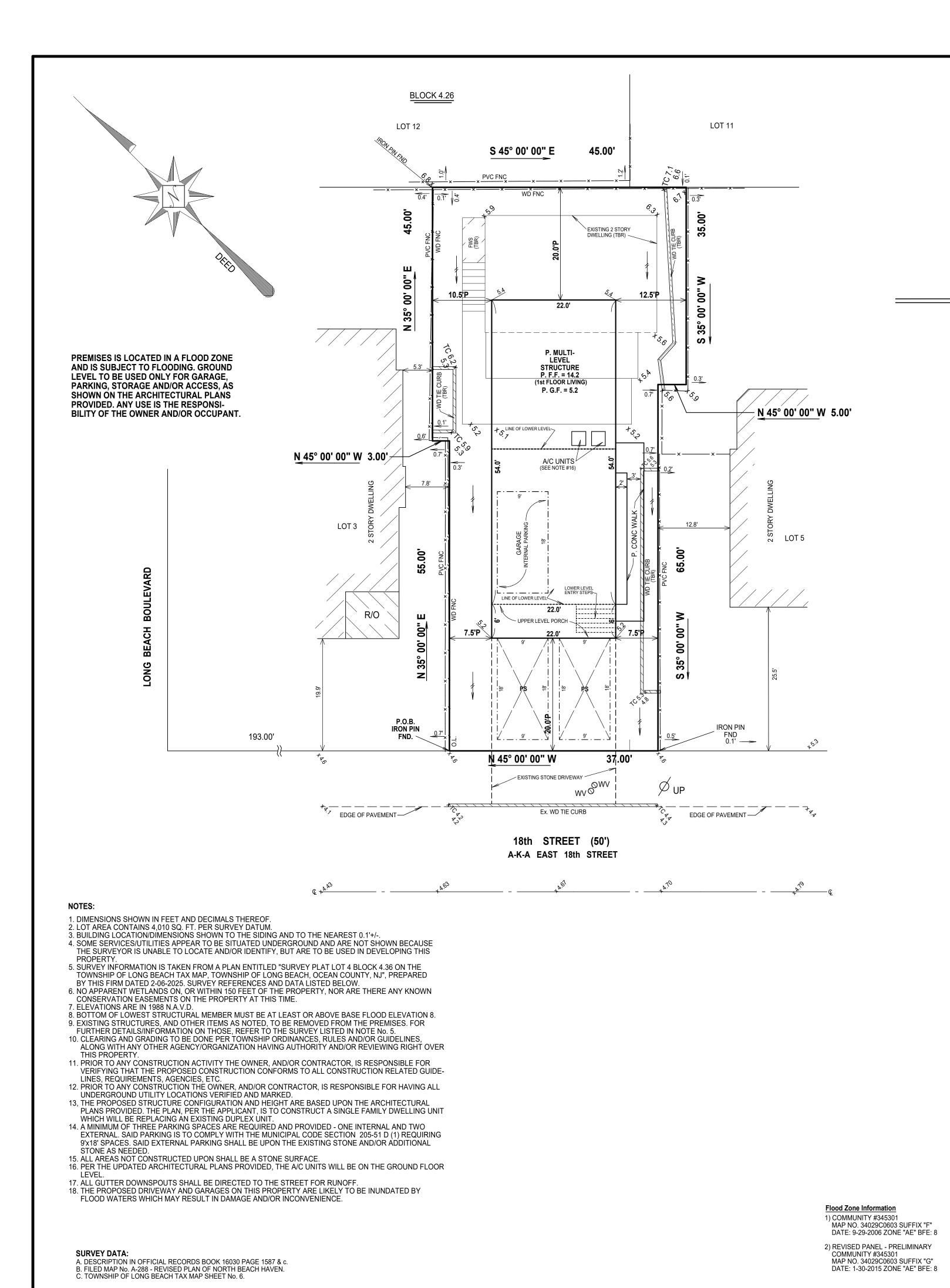
LEGEND ...POINT OF BEGINNING ...CENTER LINE .MORE OR LESS ....EXISTING SPOT ELEVATION ...PROPOSED SPOT ELEVATION ..FINISH FLOOR .GARAGE FLOOR ..EXISTING PROPOSED ...FLOW ARROW ...WOOD ...FENCE TOP OF CURB ..UTILITY POLE ...WATER VALVE ....TO BE REMOVED ....FOOT WASH STATION PS ...... CONC .. R/O ..... ...PARKING SPACE .....CONCRETE .....ROOF OVER
