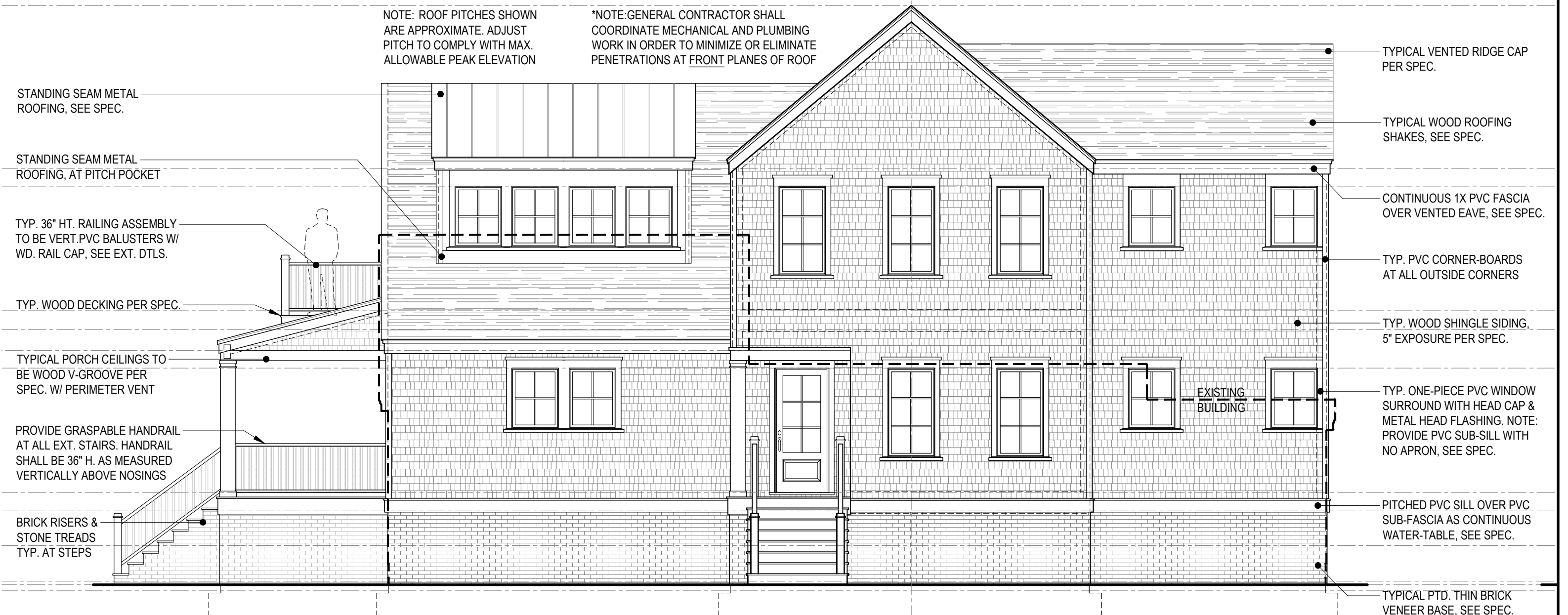
4 FRONT ELEVATION (SOUTH) SCALE: 3/16" = 1'-0"
