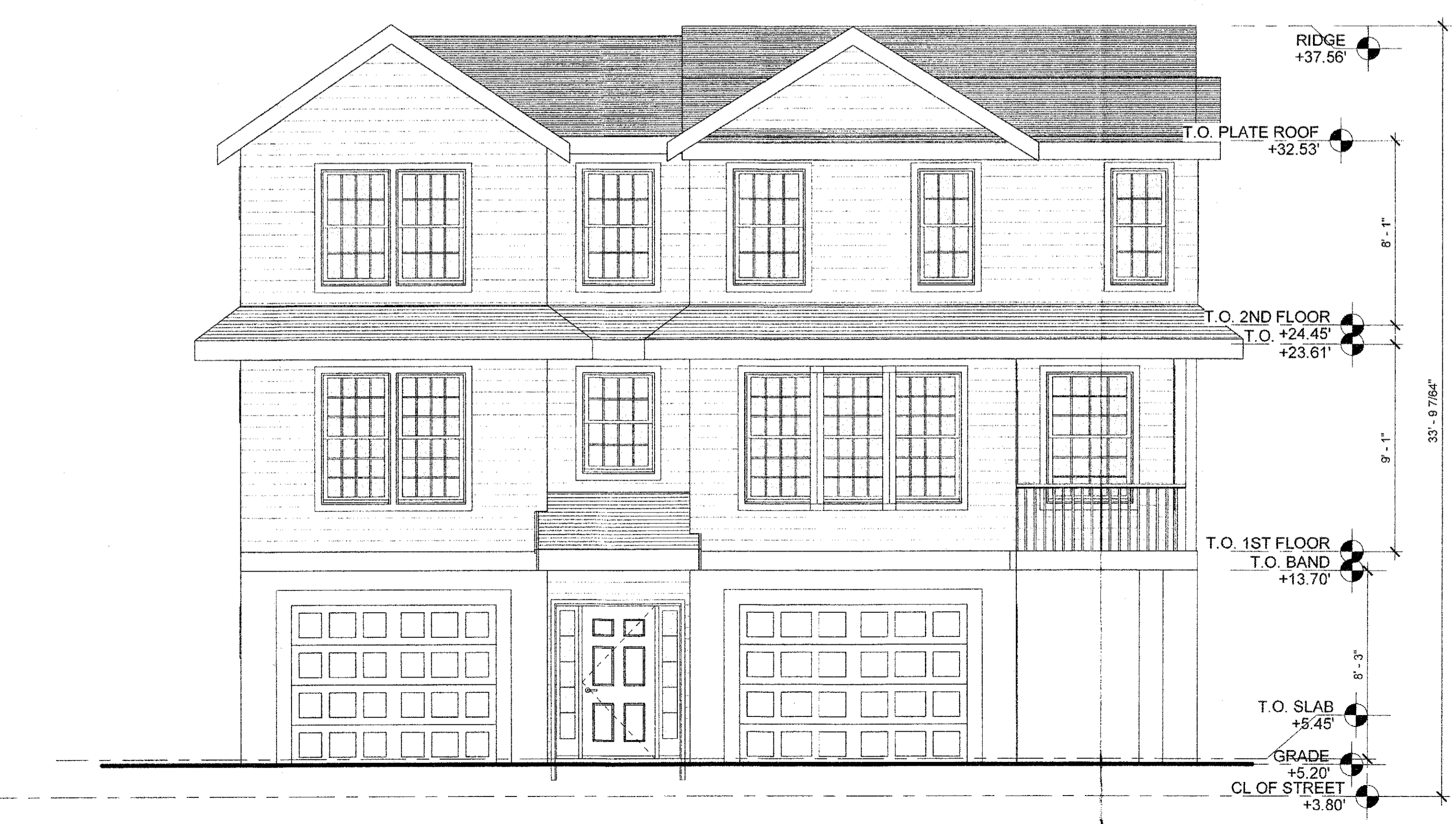
FRONT - BEACH AVE - EAST ELEVATION 1/4" = 1'-0"
